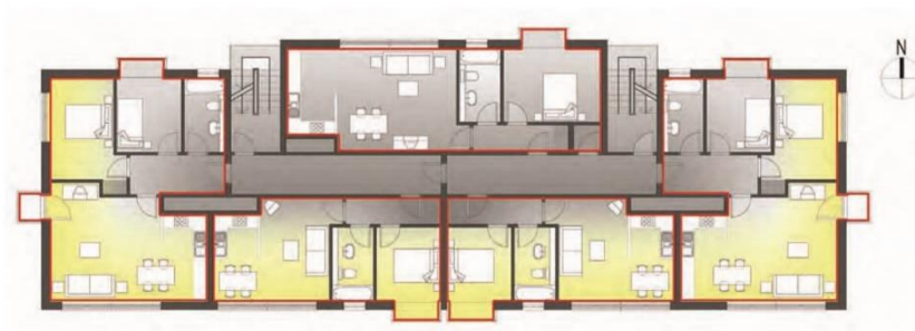
Figure 26: Careful layout design means that four out of the five flats shown have a south-facing living room
